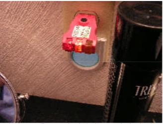
polarity is noted. Basement bathroom. Reversed polarity in an outlet is simply the improper connection of wires to the outlet itself, and is easily correctable. Because of the nature of this work however, I suggest you leave the repair to a licensed electrician. Some electronic appliances sustain damage when connected to reversed polarity outlets.
